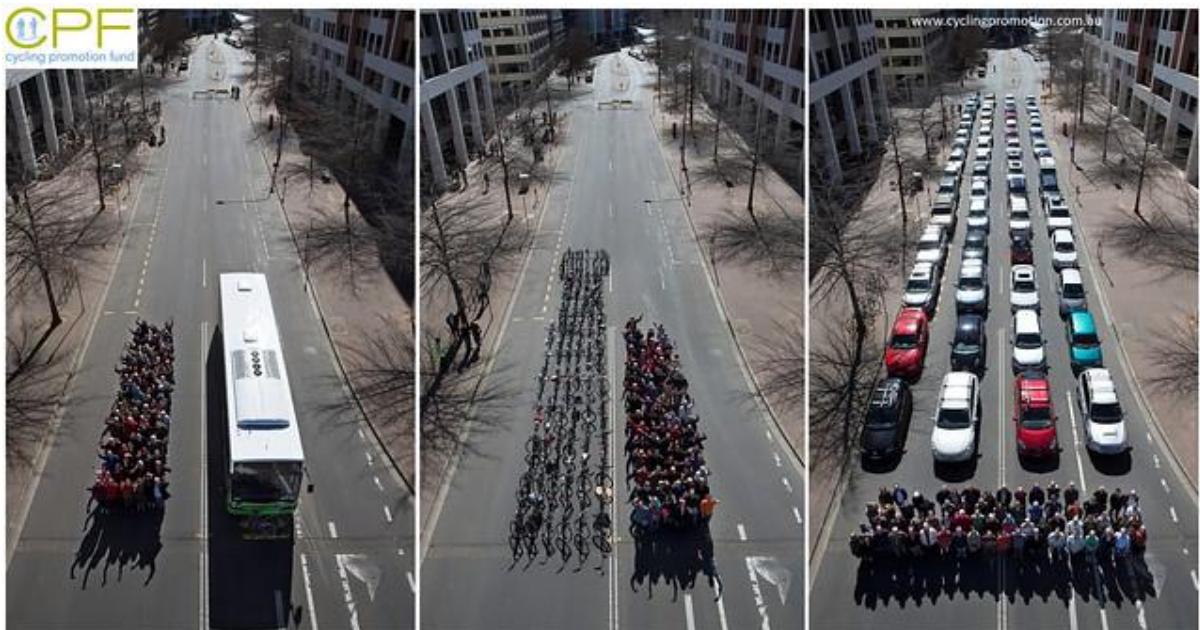
Figure 73. Road space taken up by 69 bus passengers, cyclists, and car passengers. Source: Cycling Promotion Fund
